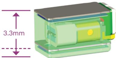
**NEW DUAL-DIAPHRAGM RLQ DELIVERS BEST-IN-CLASS OUTPUT FOR SIZE**
